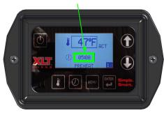
3 **BELT TIME ADJUST**: Press TIME button for three (3) seconds. To adjust belt time use either the Up or Down arrow until desired belt time is displayed and then press Enter
