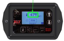
2 TEMPERATUE ADJUST: Press TEMP button for three (3) seconds. To adjust temperature use either the Up or Down arrow until desired temperature is displayed and then press Enter
