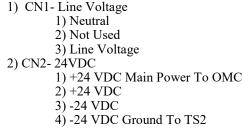
PS - The Power Supply rectifies line voltage to 24 VDC, and supplies power to the OMC.
