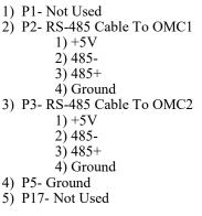
**LUI** - The Large User Interface is powered by +5 VDC from the OMC via the RS-485 cable. The main power button is located on the front face of the LUI. The conveyor(s) and temperature of the oven is controlled through the LUI. The LUI and OMC communicate via the  $485\pm$  on the RS-485 cable. The LUI will display error messages and maintenance alarms. There are twelve (12) menu presets for predetermined time and temperature settings. The screen can be locked to prevent unwanted changes.
