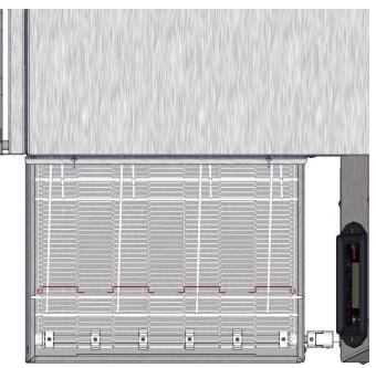
(2) Using Needle Nose Pliers, remove the Master Links.
