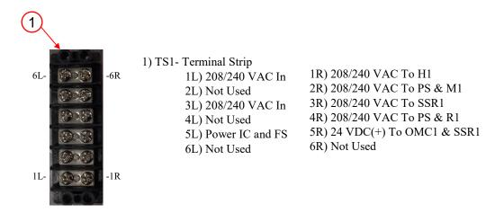
TS 1 - The terminal strips serve as a connection point for wires to and from multiple components.
