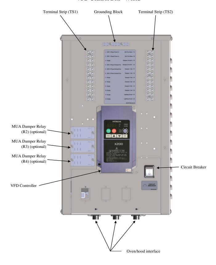
VFD Control Box (Cover removed)
