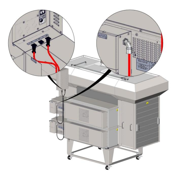
All hoods are outfitted with three (3) control cord outlets, regardless of how many XLT Ovens are installed. For a single oven use "Top" location. For a double stack use "Top" location for upper oven and "Bottom" location for lower oven, leaving "Middle" location open.
