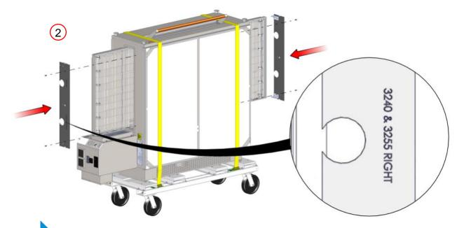
The Lifting Pipe hole, marked for the appropriate oven size, must be installed closest to the control box.
