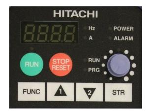
Put controller into display mode by pressing the <FUNC> button and holding until d001 appears on the display release and then press the <FUNC> button one time. The display should show 0.0.
