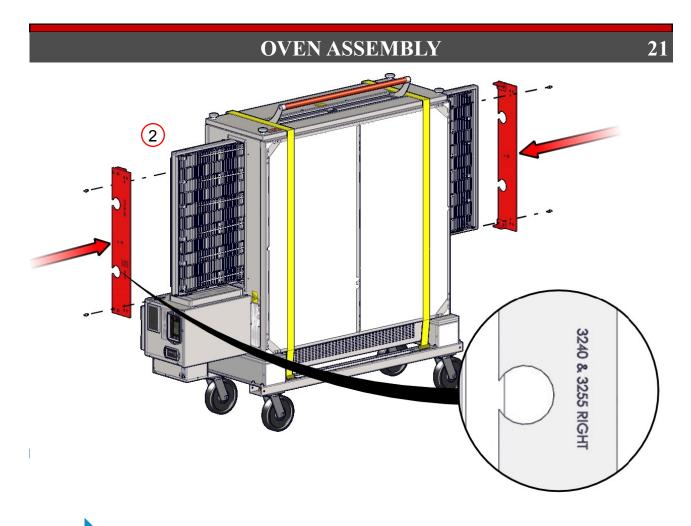
The Lifting Pipe hole, marked for the appropriate oven size, must be installed closest to the control box.
