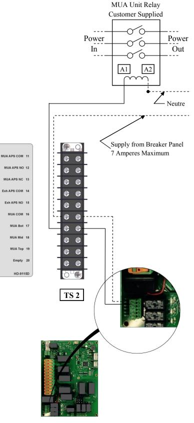
Some wiring removed for clarity. See schematic for details.
