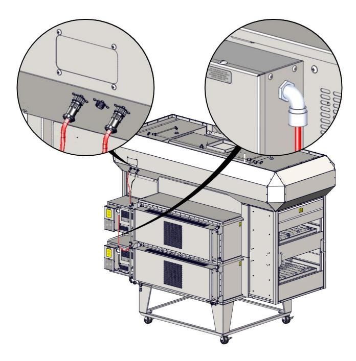
All hoods are outfitted with three (3) switch relocation receptacles, regardless of how many XLT Ovens are installed. For a single oven use "Top" location. For a double stack use "Top" location for upper oven and "Bottom" location for lower oven, leaving "Middle" location open.
