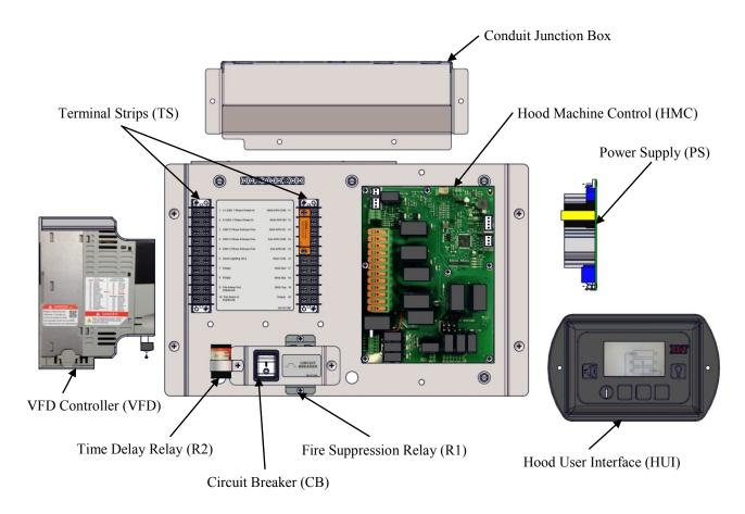
VFD Control Box (Cover removed)
