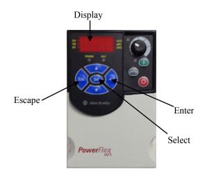
With the Oven Control switched off and power connected to the oven, the VFD should show 0.0 on the display.
