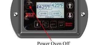
Press TIME button for 3 seconds. To adjust belt time use either the UP or DOWN arrow. If split belt press the TIME button to change to other time. Press ENTER to save.
