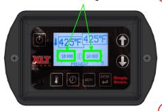
(3) BELT TIME ADJUST: Press TIME button for three (3) seconds. To adjust belt time use either the Up or Down arrow. If split belt, press the TIME button to toggle between belt times. Press Enter to save.
