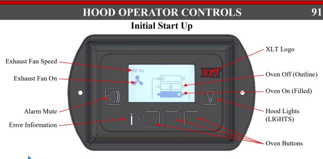
NOTE When XLT Ovens are outfitted with an XLT Hood and the receptacles unplugged from the wall and plugged into the hood., the main switch on the oven is disabled and no longer operates. The Hood User Interface (HUI) on the XLT Hood overrides the oven switch.
