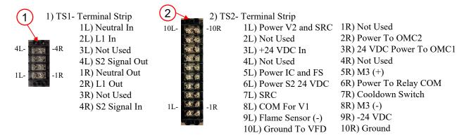
TS 1 & 2- These are terminal strips, that serve as a connection point for wires.
