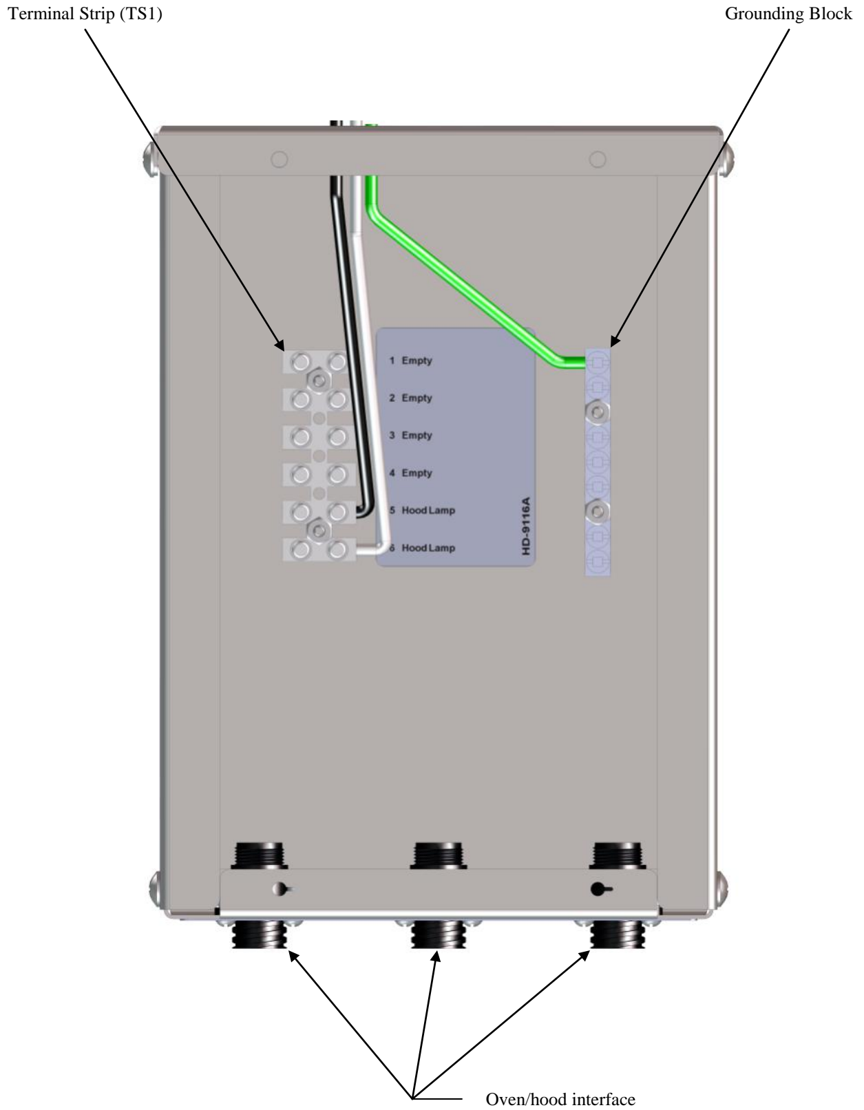
Non-VFD Control Box (Cover removed)
