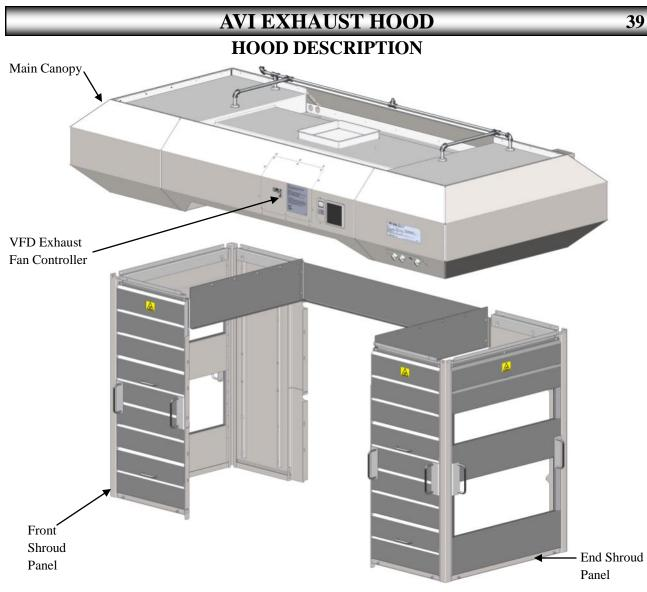
The AVI Hood System consists of three (3) major parts; the Main Canopy, the Shrouds, and the Variable Frequency Drive (VFD) exhaust fan controller.
