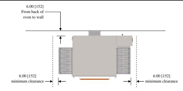
Utilities must be easily accessible when the ovens are in the installed position. Do not install utilities behind the ovens.
