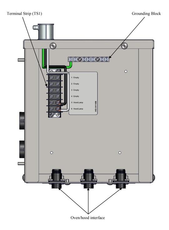
Non-VFD Control Box (Cover removed)
