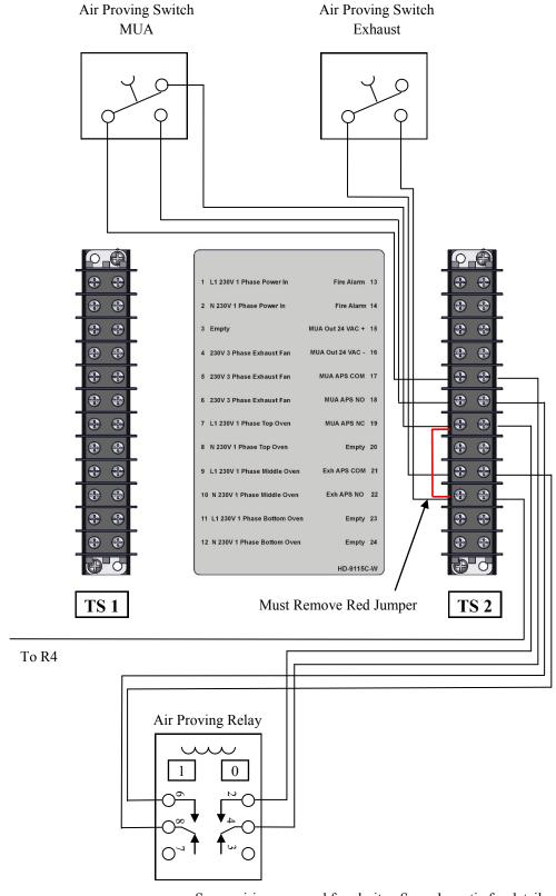
Some wiring removed for clarity. See schematic for details.
