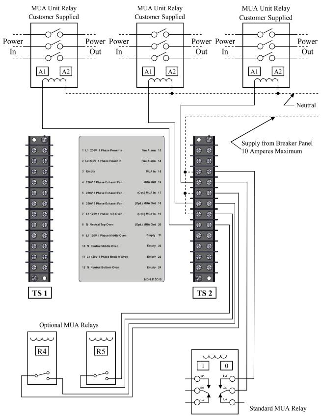
Some wiring removed for clarity. See schematic for details.
