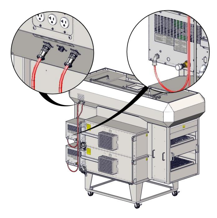
All hoods are outfitted with three (3) switch relocation outlets, regardless of how many XLT Ovens are installed. For a single oven use "Top" location. For a double stack use "Top" location for upper oven and "Bottom" location for lower oven, leaving "Middle" location open.
