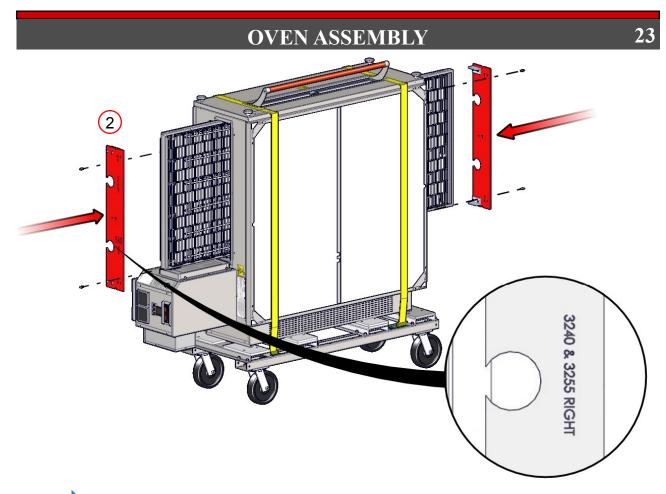
The Lifting Pipe hole, marked for the appropriate oven size, must be installed closest to the control box.
