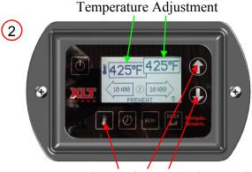
Press TEMP button for 3 seconds. To adjust temperature use either the UP or DOWN arrow. If double burner press the TEMP button to change to other temp. Press ENTER to save.
