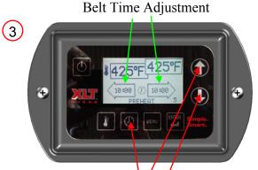
Press TIME button for 3 seconds. To adjust belt time use either the UP or DOWN arrow. If split belt press the TIME button to change to other time. Press ENTER to save.
