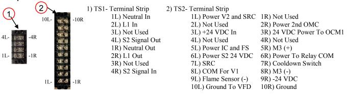
TS 1 & 2- These are terminal strips, that serve as a connection point for wires.
