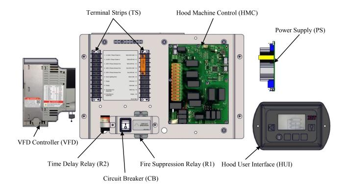
VFD Control Box (Cover removed)
