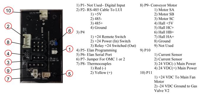
**OMC** - The Oven Machine Control reads selections or parameters from the LUI. It holds the logic for the conveyor controls and the temperature controls. The OMC will turn on or off V2, start and stop M1, send the call for heat signal, reads the thermocouple and monitor the current sensor.
