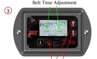
Press TIME button for 3 seconds. To adjust belt time use either the UP or DOWN arrow. If split belt press the TIME button to change to other time. Press ENTER to save.
