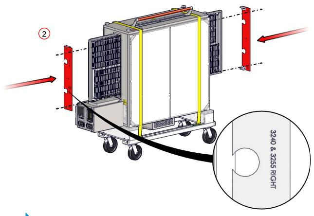
The Lifting Pipe hole, marked for the appropriate oven size, must be installed closest to the control box.
