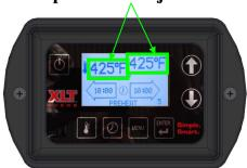
TEMPERATUE ADJUST: Press TEMP button for three
