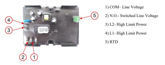
**S3 - World Ovens-** The High Limit Switch is an electronic, SPST switch. Its purpose is to provide fail safe operation. If the RTD temperature exceeds  $650^{\circ}F/343^{\circ}C$  the red LED will turn off and S3 opens to interrupt line voltage to all components. In order to reset the S3, you must unplug the main power supply.
